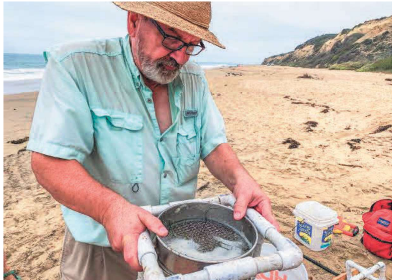
THE HUNT: During a microplastics survey at Crystal Cove State Park, a tape measure (photo far left) is used to transect a 100-meter section of beach at the high-tide wrack line on Feb. 26, 2022. Along that transect, random 20-by-20-inch squares are scraped of sand, 2 inches deep. Dr. Mark McReynolds (photo above) sifts collected sand through a sieve that surfaces microplastics, such as the white nurdle seen on his fingertip (photo left).
